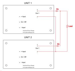
The ratings of Dx should be 1.5 times the maximum current and voltage expected in each branch.
