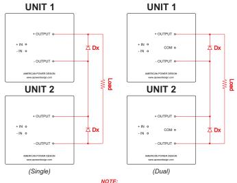
The ratings of Dx should be 1.5 times the maximum current and voltage expected in each branch
