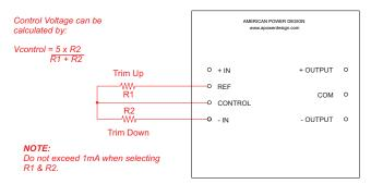
The figure below shows how to adjust the output voltage using an external Trim Pot.
