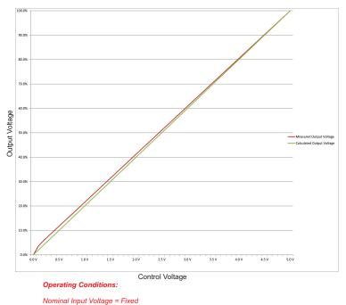
Output Load = Resistive (fixed at full output current @ 100% output voltage)
