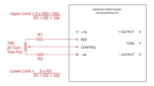
Figure below shows how to remotely mechanically shutdown the converter while maintaining any preset control voltage.
