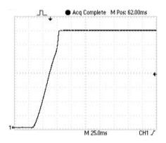
Figure below shows a typical output voltage during turn-on, measured at full rated load current with no additional output filtering.
