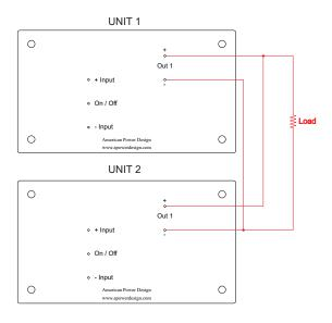
The figure below show how to connect several dual output units with equal nominal output voltage in parallel.
