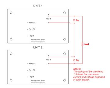
Figure below shows how to connect multiple dual output units in series with the use of shunt diodes.
