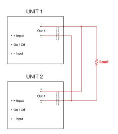
The figure below shows how to connect several dual output units with equal nominal output voltage in parallel.
