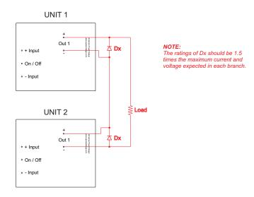
Figure below shows how to connect multiple dual output units in series with the use of shunt diodes.
