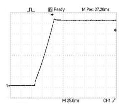
Figure below shows a typical output voltage during turn-on, measured at full rated load current with no additional output filtering.
