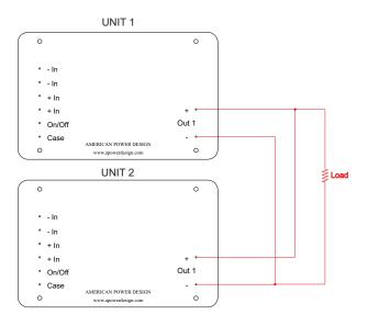
The figure below shows how to connect several dual output units with equal nominal output voltage in parallel.
