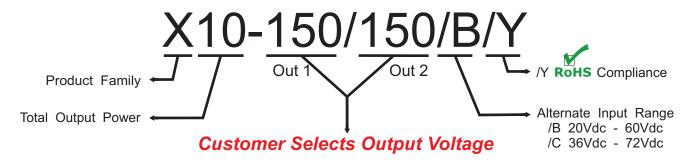
The X10 Series are designed such that the customer may order any output voltage from 24Vdc to 500Vdc at no additional charge.
