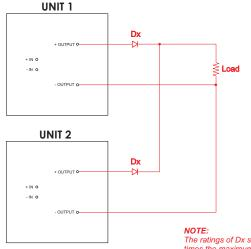
**NOTE:** The ratings of Dx should be 1.5 times the maximum current and voltage expected in each branch.
